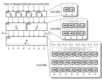
Fig. 4. Block diagram of an 8-bit enhanced bitonic-sorting network, showing also the structure of the corresponding 2-, 4-, and 8-bit EBS units.
