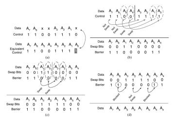
Fig. 8. Example of the functionality of the 8-bit EMS.
