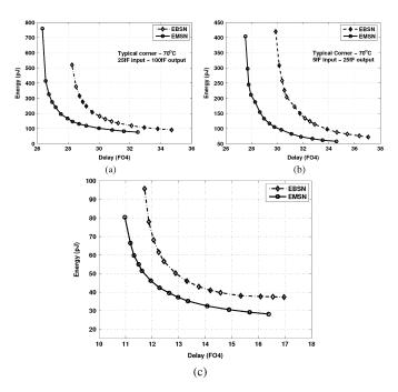
Fig. 10. Energy-delay curves for the 64-bit GRP units implemented with the EBSN and EMSN, respectively, (a)  $C_{\rm in}/C_{\rm out}=25/100$  fF and (b)  $C_{\rm in}/C_{\rm out}=5/25$  fF. (c) The energy-delay curve for a subword oriented GRP unit that supports a minumum subword size of 1 byte.
