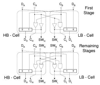
Fig. 6. Implementation of the HB and LB cells.
