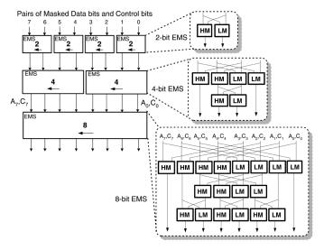
Fig. 7. 8-bit enhanced merge-sorting network and the structure of the 2-, 4-, and 8-bit EMS units.
