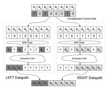
Fig. 3. Implementation of GRP using two separate extraction units.
