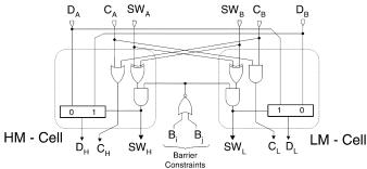
Fig. 9. Implementation of the HM/LM cell used in all stages of the EMS following the first.
