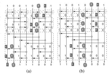
Fig. 2. 8-bit sorter designed using (a) a bitonic and (b) a merge-sorting network.
