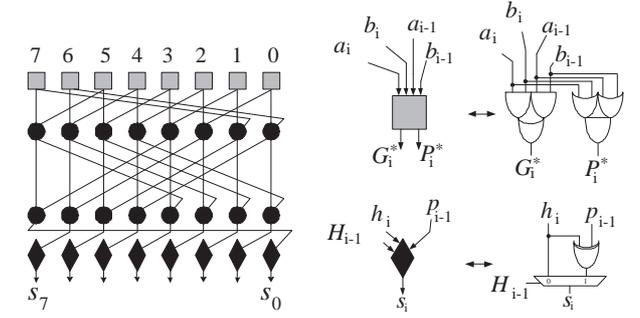
**Figure 6.** The proposed Ling-based modulo  $2^8 - 1$  adder and the definition of the new preprocessing and sum bits computation stages.
