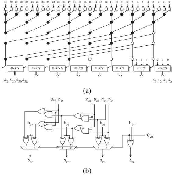
**Figure 2.** (a) Sparse-4 parallel-prefix structure for a 32-bit integer adder and (b) the logic level implementation of the CS block.
