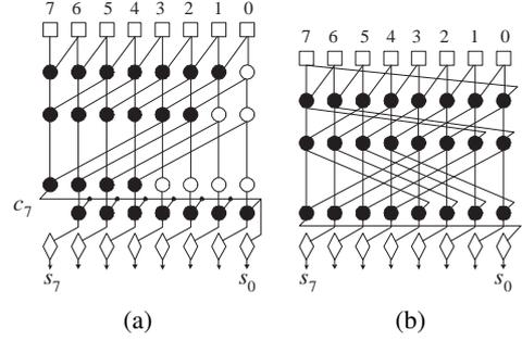
**Figure 3.** Modulo  $2^8 - 1$  adder designs.
