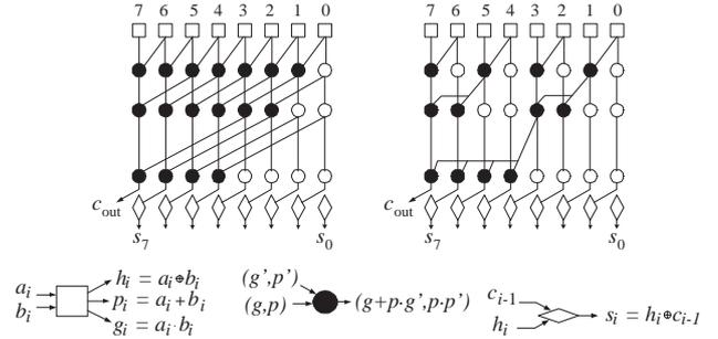
**Figure 1.** Examples of parallel-prefix structures for integer adders.
