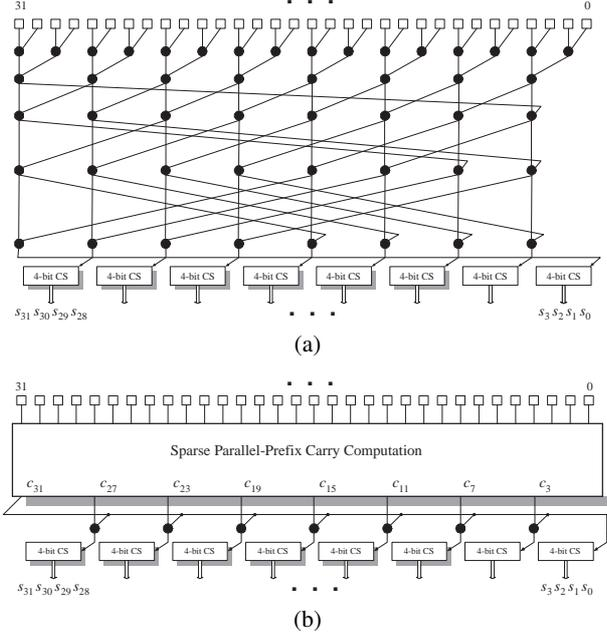
**Figure 5.** The proposed 32-bit sparse modulo adders using the architectures of [6] and [5], respectively.
