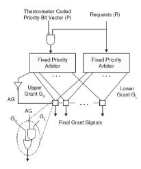
Fig. 3. The dual-path arbiter proposed in [12].
