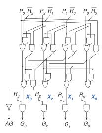
Fig. 5. Fast 4-bit arbiter.
