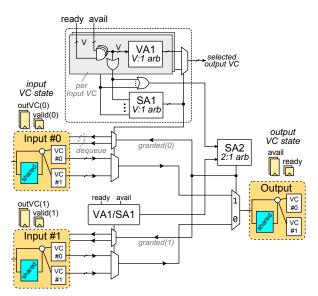
Fig. 4. The fundamental ElastiNoC primitive, the Merge Unit (MU). The diagram depicts the per-input and per-output multiplexers together with the combined allocation logic (SA1, SA2) that runs in parallel to VA1.
