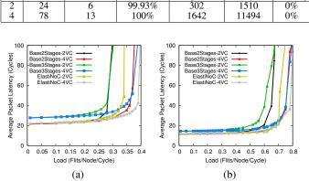
Fig. 8. Latency vs. load curves for (a) uniform random traffic and (b) nonuniform localized traffic. Network traffic from real applications is estimated to lie in-between these two synthetic traffic patterns.
