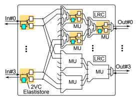
Fig. 3. The modular construction of an example ElastiNoC  $4 \times 4$  VC-based router using the proposed MU primitive that supports 2 VCs.
