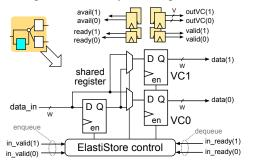
Fig. 5. The ElastiStore-based buffer architecture. ElastiStore consists of merely one single-flit register per VC, plus one additional single-flit register that is shared dynamically between VCs.
