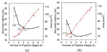
Fig. 2. The average zero-load packet latency (in absolute time) computed directly from eq. (3) and the associated router area overhead, as the number of pipeline stages are varied. Results are shown for (a) a baseline, and (b) a speculative VC-based router assuming 4 VCs per input port.
