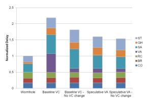
Fig. 1. The delay of representative single-cycle 5-port NoC routers with 64-bit wide ports and 4 VCs per input in the case of VC-based routers. The results are normalized to the delay of a wormhole-based router (i.e., no VC support). "No VC change" means that packets do not change VC; their VC is decided upon injection and remains the same until they reach their destination.
