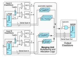
Fig. 6. BIST enhancements of a merge unit by incorporating the logic of LSFR/MISR within that of the shared buffer at each ElastiStore.
