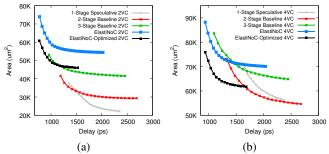
Fig. 7. Hardware implementation results of various router designs with (a) 2 VCs, and (b) 4 VCs per port.
