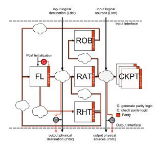
Fig. 3. The proposed Circular Parity (CP) protection scheme. Parity generation ('G') is performed at only one location (during initialization), and parity checking ('C') at two locations (at the output of the RRS).
