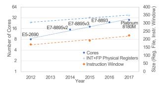
Fig. 1. Prevailing trends with technology scaling for the Intel core microarchitecture [10] and Intel Xeon processors.
