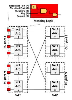
Figure 3: Packet throttling is achieved using minimal masking logic, which is placed in front of the router's Virtual-channel Allocation (VA) module. A separable VA is shown here [6].
