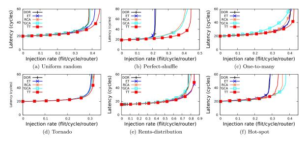
Figure 5: Latency vs. load curves for the 5 investigated designs, under various synthetic traffic patterns.
