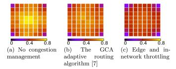
Figure 1: The average buffer utilization rate observed in the routers of an  $8 \times 8$  2D mesh NoC, with and without congestion management techniques. Lighter colors indicate higher congestion.
